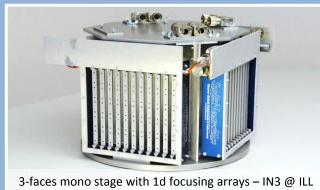
3-faces mono stage with 1d focusing arrays – IN3 @ ILL
